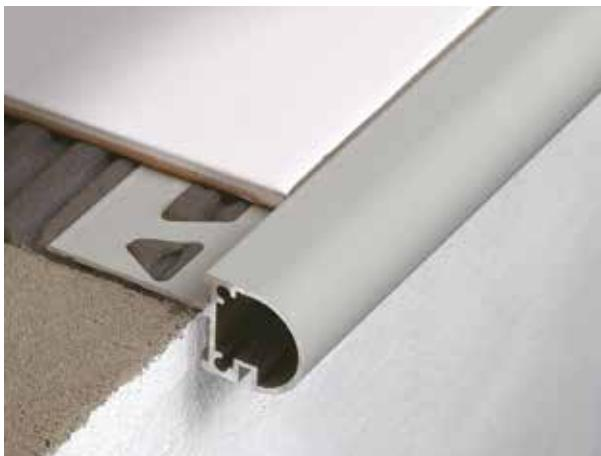
Perimeter profile that finishes and protects the exposed concrete edge of balconies and terraces incorporating a symmetrically shaped upper edging trim designed to frame the tiles surface. Particularly suitable for tiling on pre-existing floors. Includes an integrated "drip-lip". It is important to leave a space between elements for thermal expansion and covered by the covering cap.
